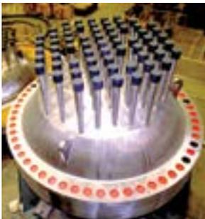
***At left: Top of nuclear reactor showing tubes for fuel and for control rods. The core of a nuclear reactor is constructed with many parallel tubes. Most of the tubes contain nuclear fuel. However, some of the tubes are left empty, so rods of cadmium can be lowered into them to absorb neutrons and control the nuclear reaction.***
