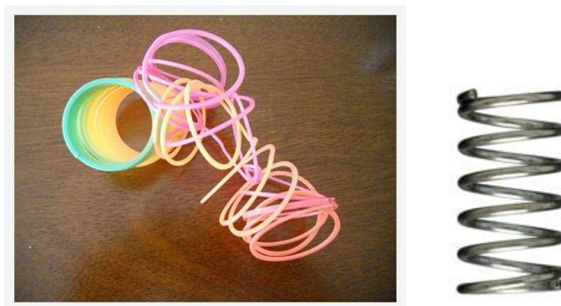
Figure 3: One of the many “folds” a Slinky can adopt (left). A metal spring (right) has very little flexibility in comparison. 3
