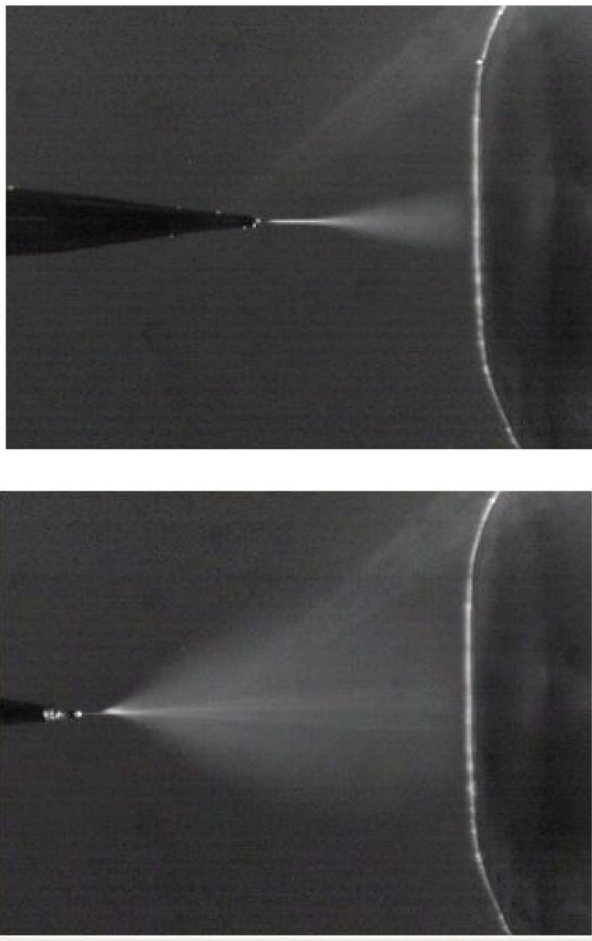
**Figure 5.** Electrospray ionization (ESI) from the tip of a capillary toward the inlet of a mass spectrometer. The opening of the tip is approximately 1-2  $\mu\text{m}$  in diameter. Formation of a single Taylor cone (top) and multiple Taylor cones (bottom). *Images courtesy of Arne Ulbrich.*
