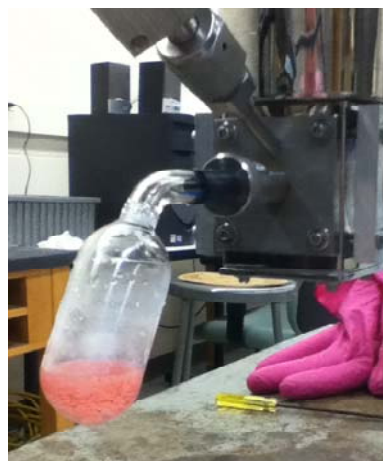
Diazo compound in a deposition tube ready to be matrix-isolated
