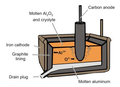
Aluminum is a silvery-white metal with many valuable properties. It is light (density 2.70 g/cm<sup>3</sup>), non-toxic, and can be easily machined or cast. With an electrical conductivity 60% that of copper and a much lower density, it is used extensively for electrical transmission lines. Pure aluminum is soft and brittle, but can be strengthened by alloying with small amounts of copper, magnesium, and silicon.
