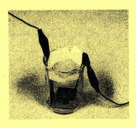
Attach a clip from one wire to the copper. Attach a clip from a different wire to the zinc.
