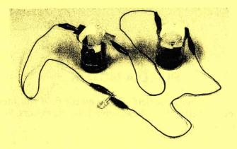
Gently and slowly move your battery close enough to your neighbor's to connect the two with one of the clip wires. Clip the wire from the zinc in one battery to the copper in the other battery.
